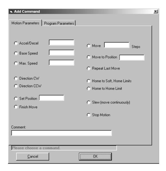
The motion command tab sheet controls the motion information of the motor such as Acceleration/ Deceleration, Maximum Speed, Base Speed, Move number of Steps, and etc.
